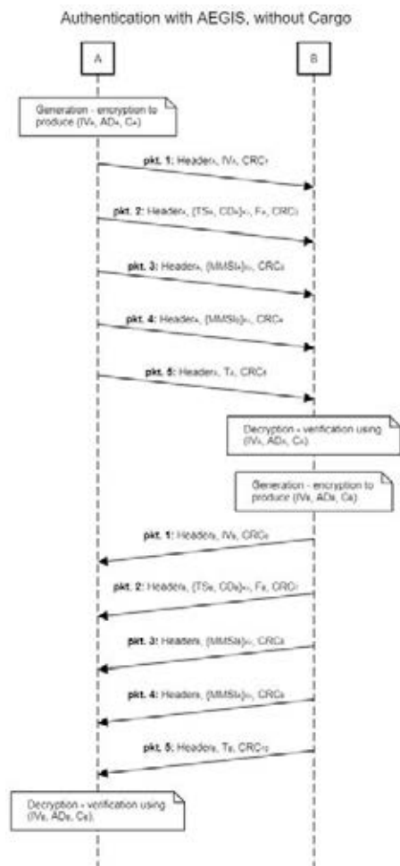
Figura 4. AEGIS used in authentication protocol, without usage of cargo.
